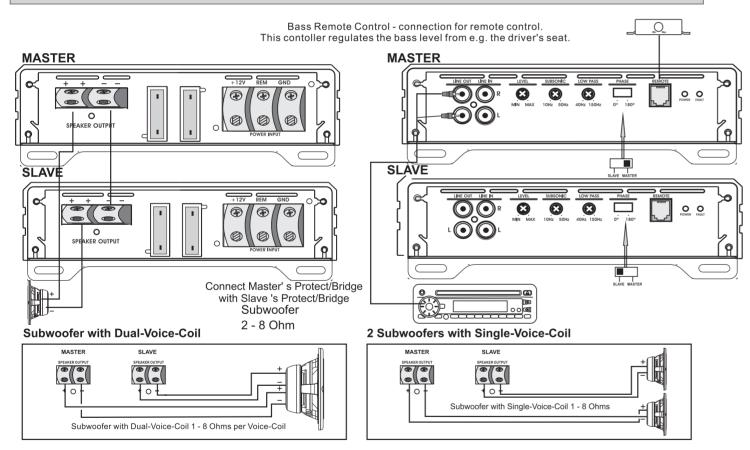
$Caution: Please \ observe \ the \ right \ polarity. \ Slave's - to \ Loudspeaker's + and \ Slave's + to \ Loudspeaker's - to \ Loudspeaker's + and \ Slave's + to \ Loudspeaker's - to \ Loudspeaker's + to \ Loudspeaker's - to \ Loudspeaker's + to \ Loudspeaker's - to \ Loudspeaker$
