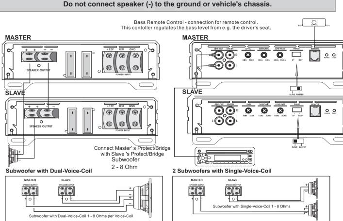
${\tt Caution: Please \ observe \ the \ right \ polarity. \ Slave's - to \ Loudspeaker's + and \ Slave's + to \ Loudspeaker's - to \ Loudspeaker's + and \ Slave's + to \ Loudspeaker's - to \ Loudspeaker's + and \ Slave's + to \ Loudspeaker's - to \ Loudspeaker's + and \ Slave's + to \ Loudspeaker's - to \ Loudspeaker's + and \ Slave's + to \ Loudspeaker's - to \ Loudspeaker's + and \ Slave's + to \ Loudspeaker's - to \ Loudspeaker's + to \ Loudspe$
