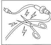
DO NOT cut or modify any DIN cables with fuse built-in. This could render such protective circuit inactive and potentially result in permanent damage to the unit or vehicle. Make sure both DIN cable and other wiring is not run where it may be cut or damaged.
