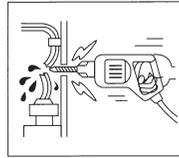
Inspect any vehicle areas before drilling any holes for mounting or wiring of unit. Make sure to check behind installation area to prevent damaging any existing vehicle wiring or other connections. Failure to do so could result in vehicle malfunction or impaired vehicle operation.
