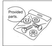
Use provided parts. Over-sized hardware may cause an electrical short or result in product not being mounted securely.
